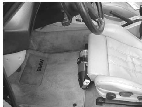
Fig 2: Fire Extinguisher and Positioning
