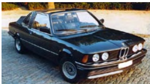
E21. Baur. Many smaller BMW's had the Baur option. It basically featured regular saloon sides with a soft roof and back window. There are a few E30's running around town. Keep an eye open.
